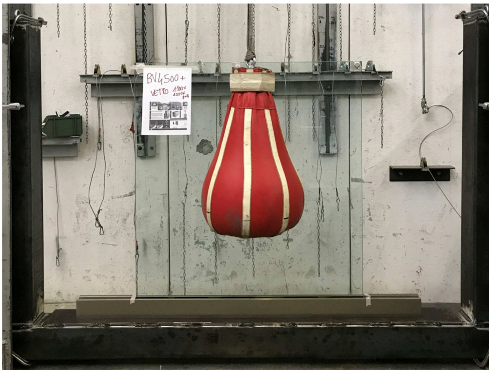
Photograph of the item after impact on the centre of the glazing with dynamic load
