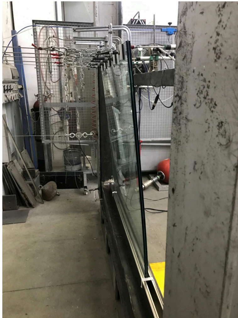
Photograph of the item undergoing horizontal linear static load
