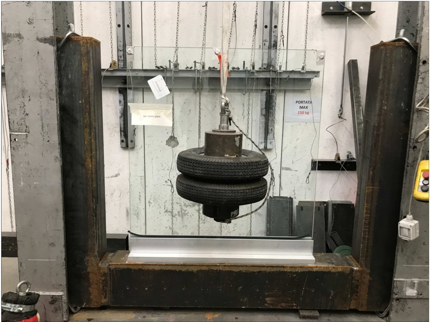
Photograph of the item after impact on the centre of the glazing according to standard UNI EN 14019:2016
