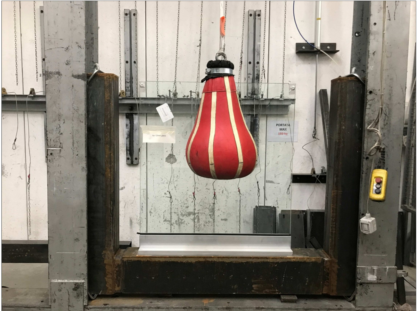
Photograph of the item after impact on the centre of the glazing according to standard NF P01-013:1988
