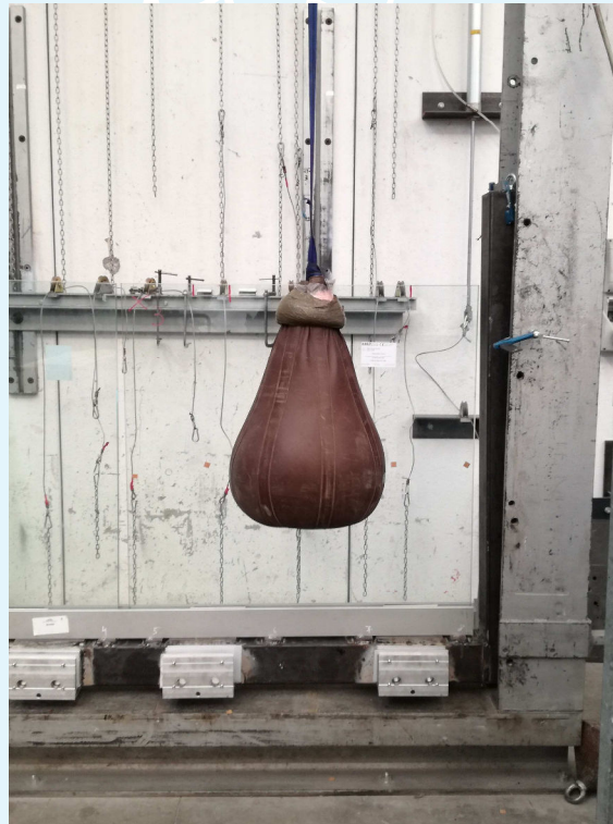
Photograph of the sample after impact in the centre of infill
