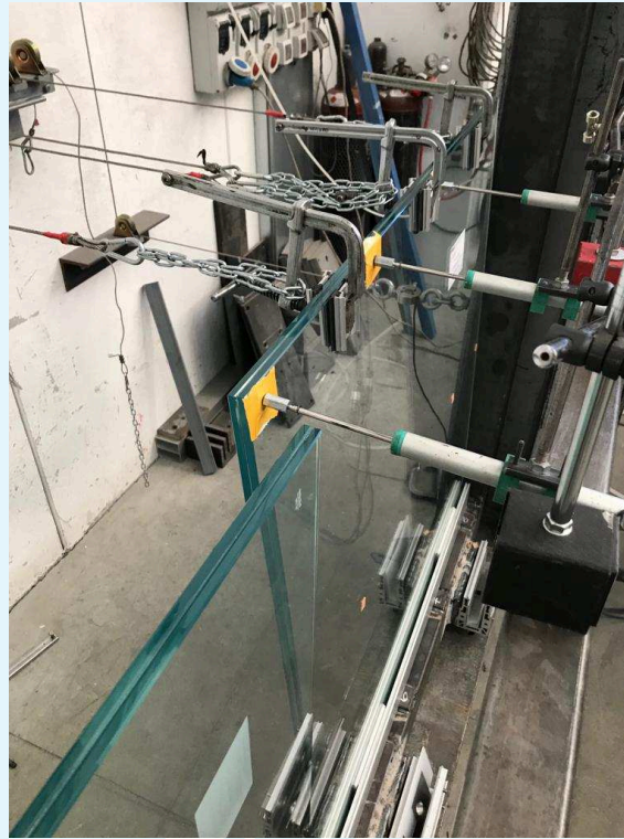
Photograph of the sample during resistance to outward horizontal static loading test
