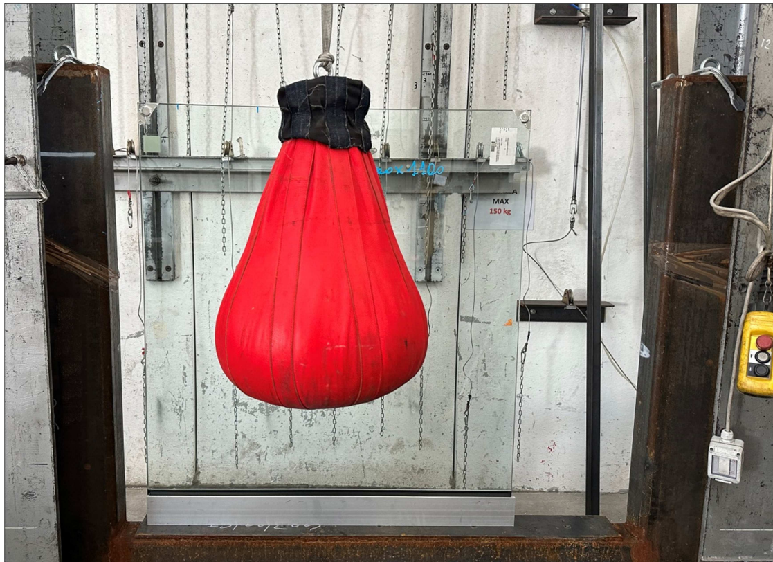
Photograph of the item after impact according to standard NF P01-013:1988
