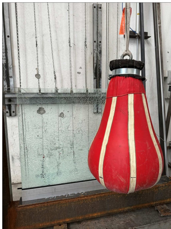
Photograph of the item after impact according to standard NF P01-013:1988
