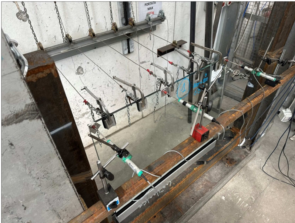
Photograph of the item undergoing horizontal linear static load
